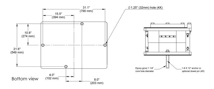
The slope of the concrete surface under the isolator must not exceed 0.07 inches/foot (5.8 mm/meter). Uneven loading of the coil springs occurs when the isolator is tilted, or twisted, causing excessive stress. Self-leveling grout or a steel plate covering the pit bottom is recommended if the supporting surface exceeds the tolerances shown above.
