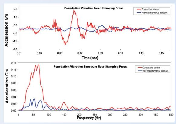
The measurements showed that the Vibro/Dynamics<sup>®</sup> Micro/Level Isolators provided an additional 80% isolation over the competitor's mounts. The customer's vibration transmission problem was solved quickly!
