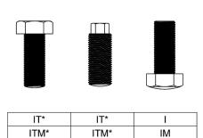
I = Leveling Screw Style T = Top Hex Option M = Metric Thread
