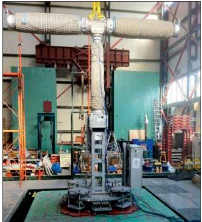
Figure 4. Physical testing setup of a circuit breaker with wire rope isolators
